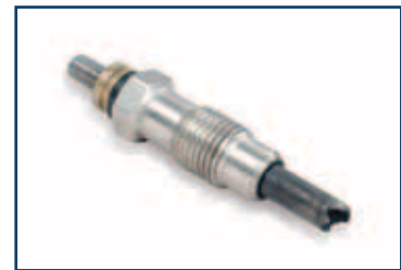
Glow Plug damaged by incorrect engine timing
