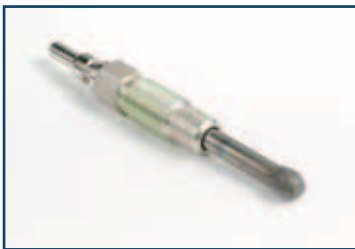
Glow Plugs damaged due to over voltage
