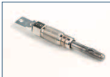
Glow Plugs damaged due to over voltage
